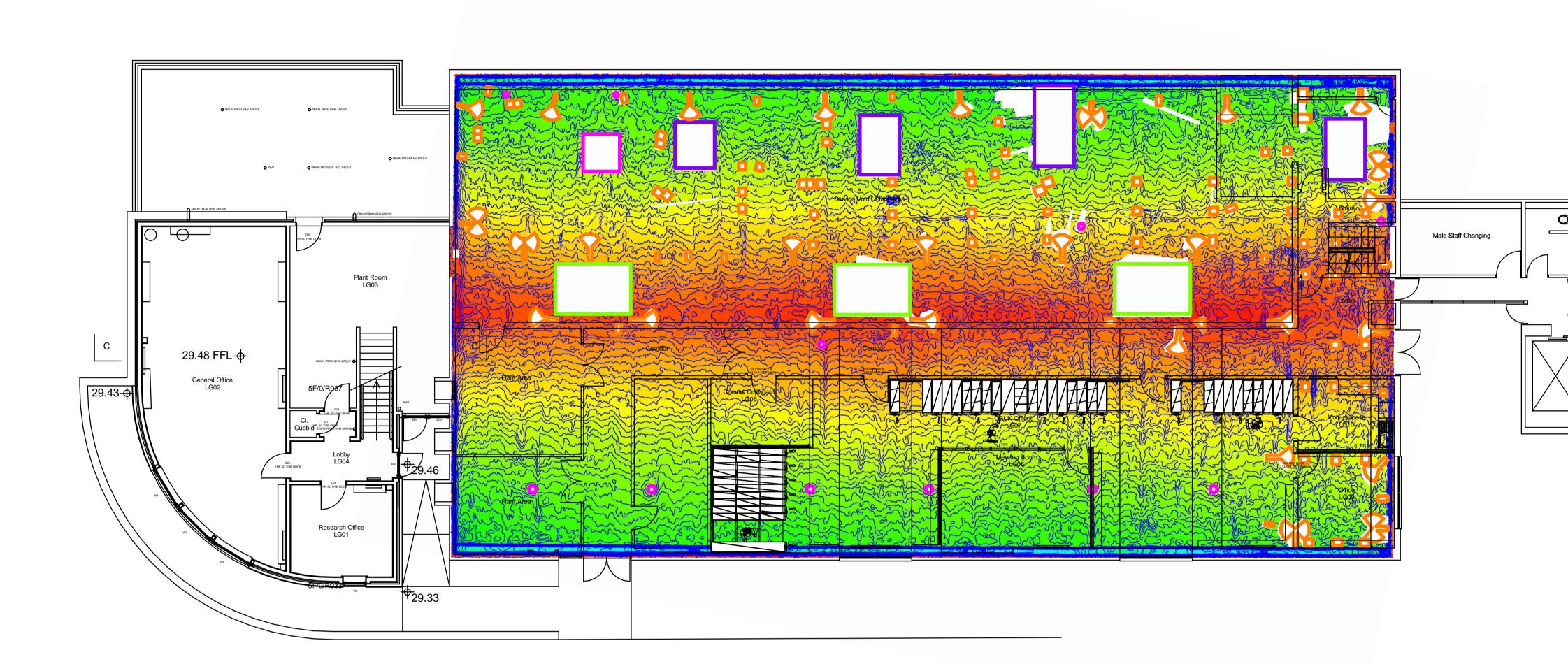
NOTE: • THE COLOURS IN THE LEGEND ABOVE INDICATE THE DISTANCE FROM DATUM UP AND DOWN WITH A RANGE OF PLUS OR MINUS 0.195m (195mm). • THE CONTOURS ARE INDICATED ON THE PLAN ARE PLUS OR MINUS 5mm.
